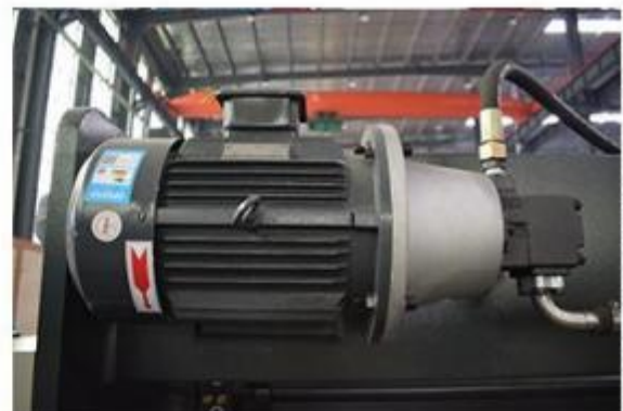
Main motor and oil pump
